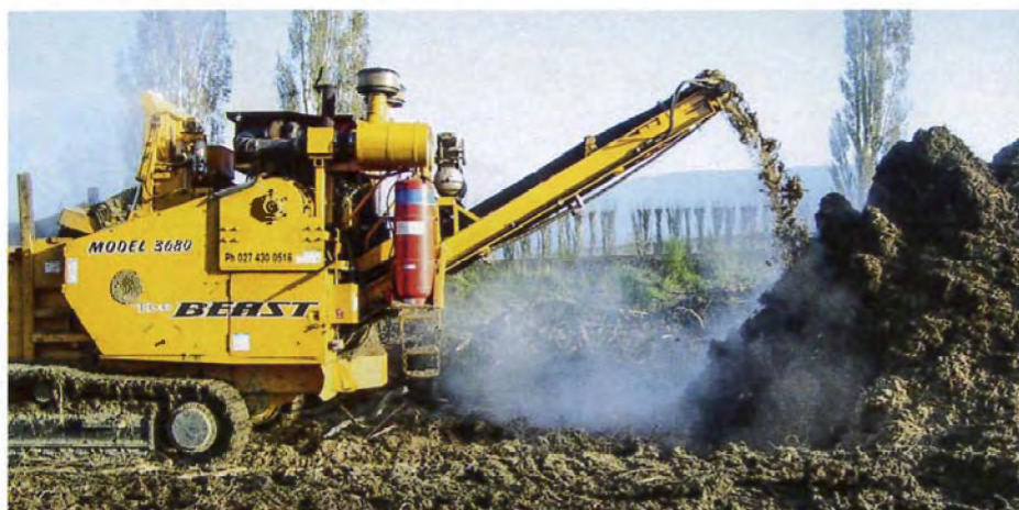
Hall Bros 'The Beast' chipper chomping on willow roots near Dunedin Airport is capable of chipping up one metre diameter logs.
