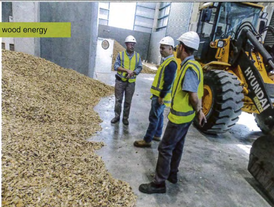
The chip bunker where wet chip is stored prior to feeding into heated chambers prior to drying for boilers is explained by Christian Jirkowsky (centre), General Manager of Polytechnik Biomass Energy, to potential buyers.
