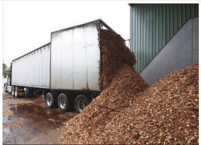
Fuel delivery onto walking floor.
